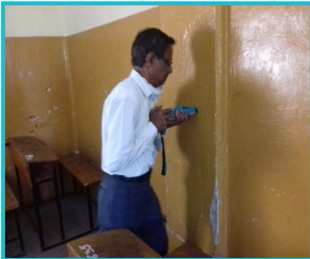
Rebound Hammer Test on Column
